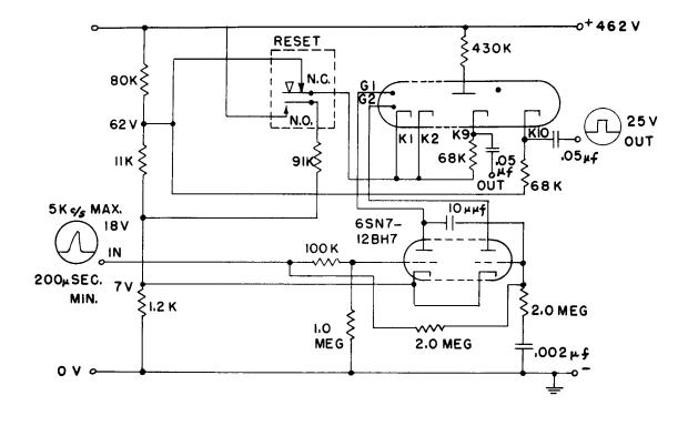
6476 GLOW TRANSFER COUNTER TUBE DRIVER CIRCUIT
