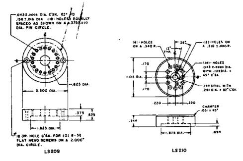
Figure 6. PIN STRAIGHTENERS
