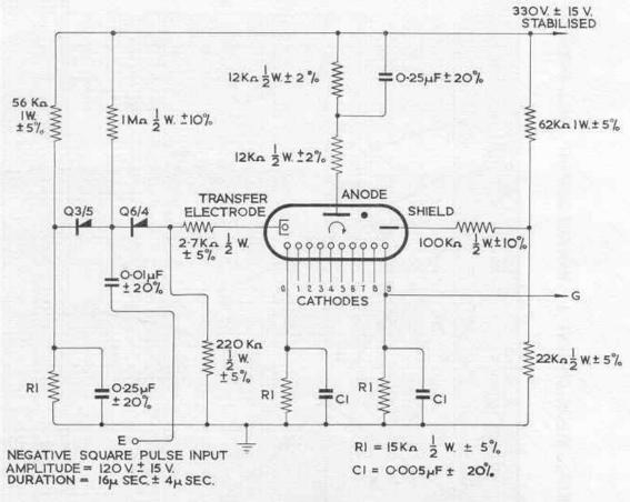
NOTE -THE CATHODE CIRCUITS OF CATHODES I TO 8 HAVE BEEN OMITTED FROM THE DIAGRAM FOR SIMPLICITY.
