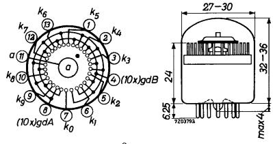
$\boldsymbol{K}_{O}$  is aligned with pin 7 to within  $\pm\,3^{O}$
